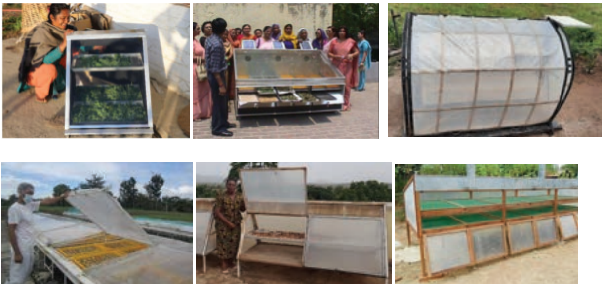
Solar dryers: Cabinet model from wood and glas (CRT, Nepal), cabinet from metal and glas (AIWC, India), Poly-Tunnel model from Bamboo, (INSEDA, India), and semi-industrial models (PHilMech) in the Philippines, and ESRITA & TaTEDO in Tanzania.
